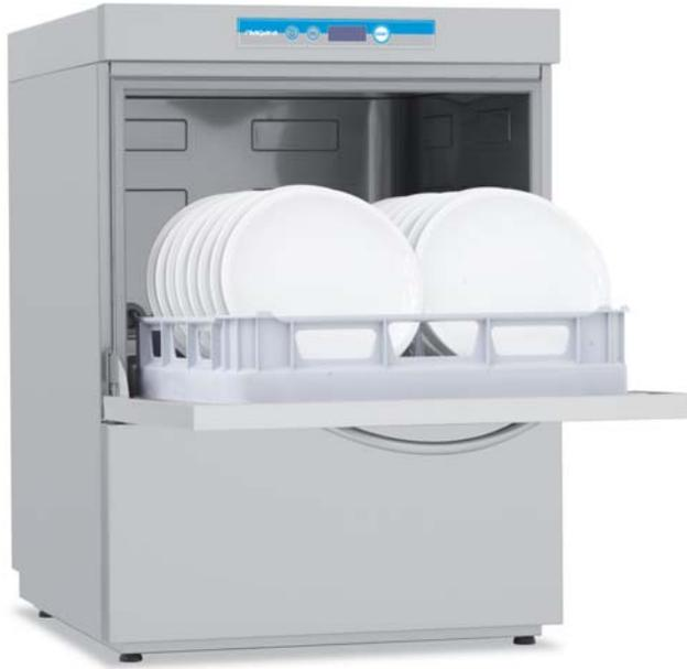
Undercounter version with 18-plate 50x50 cm rack, can also wash Gastronorm and Euronorm trays. Maximum productivity of 720 plates/hour. Useful height of 39 cm, can wash up to 35 cm high glasses. External dimensions of 60x60 cm with height limited to 82 cm permit seamless integration.
